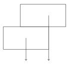
We need to place our pivot between the two arrows such that it is perfectly balanced. We know the distance between the arrows is 1m. Let x denote the distance from the pivot of the left arrow and hence 1 - x for the right. We have:
