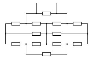
Redundant wires can be removed by symmetry:
